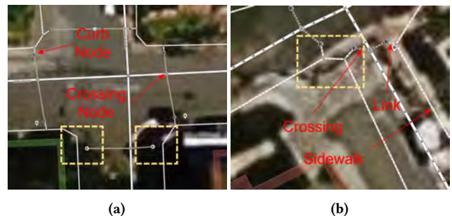
Figure 1: Example of annotations from human mappers. Red text shows different types of features in a pedestrian path network map. Yellow boxes show examples of errors made by human mapper: (a) crossing lines are not connected to the sidewalk lines with link lines (b) the curb nodes are falsely mapped to the middle of the road.
